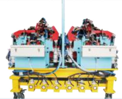
Puppet Welding jig
