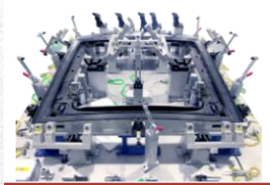
Roof assembly parts
